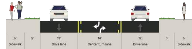
Exhibit 6.6: Minor Collector Cross Section
