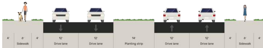
Exhibit 6.4: Minor Arterial Cross Section
