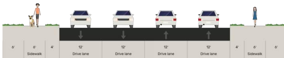
Exhibit 6.5: Major Collector Cross Section
